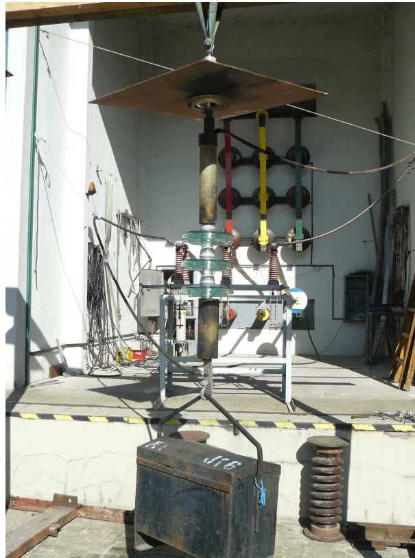
Photo 11 The test arrangement of power arc test
