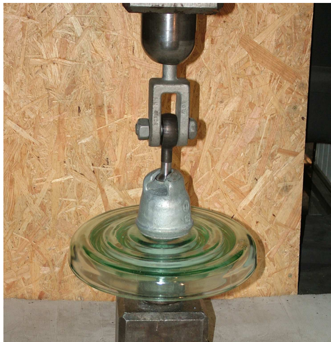
Photo 4 The test arrangement of failing load tests
