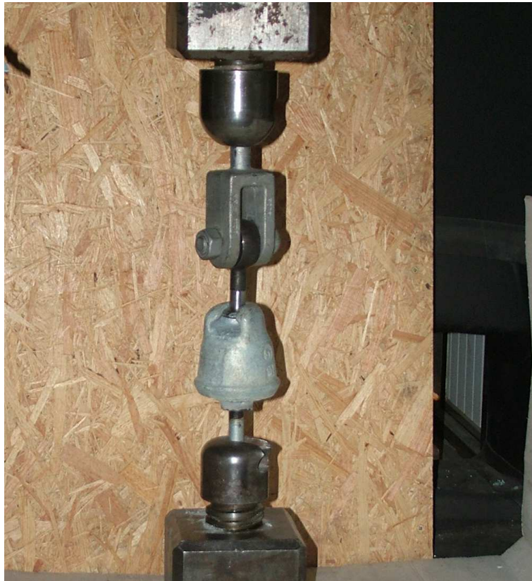
Photo 5 The test arrangement of the residual test
