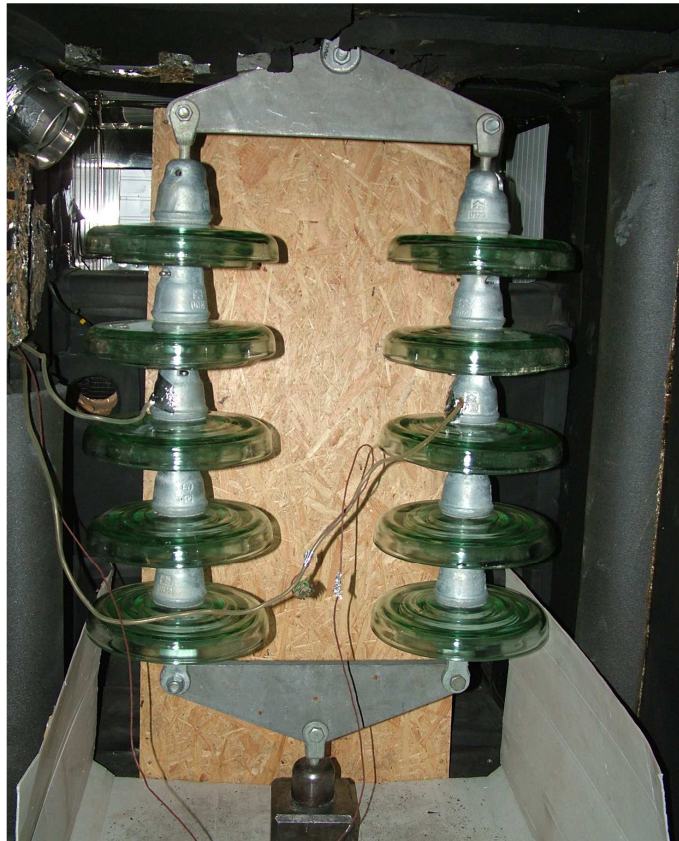
Photo 3 The test arrangement of thermal-mechanical test
