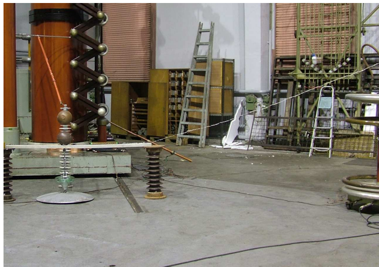
Photo 10 The test arrangement of the puncture test in air
