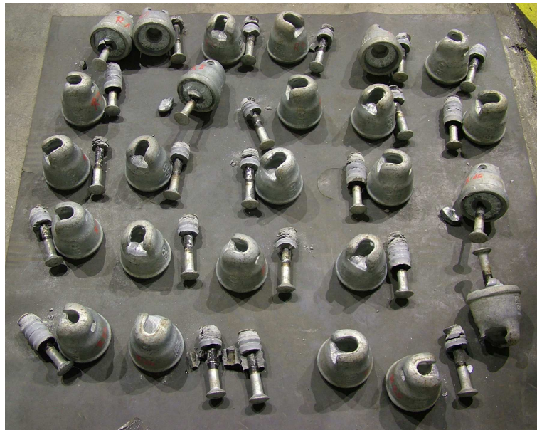
Photo 6 The broken insulators after the residual strength test
