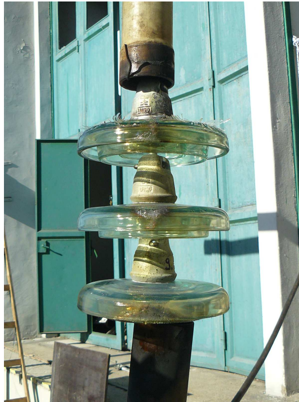
Photo 15 The third insulator string after the power arc test
